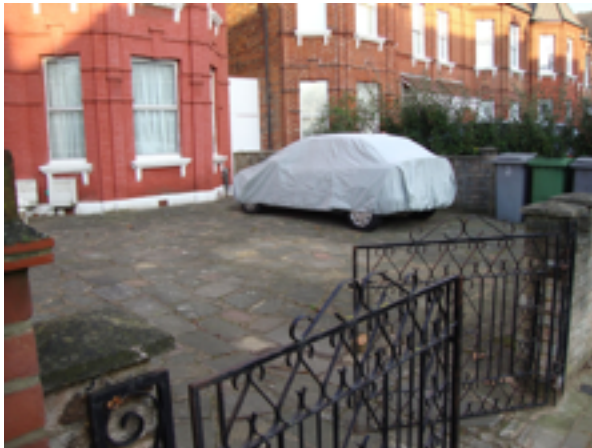
Figure 7: The front garden of this house in the conservation area of Queen's Park, London, has been paved over, without planning permission, for car parking. This increase in hard surfacing contributes to flooding, poor air quality, and the Heat Island Effect. Nearly half of London's front gardens have been paved over for car parking, an area equivalent to 22 times the size of Hyde Park.
